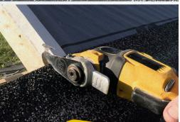
The Blaze Tool is a specialty blade designed to cut through asphalt and architectural shingles that fits on most major brands of oscillating tools.
